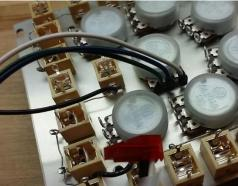
33. Create the crimped connectors for the Width pots. Wires should be approximately 3" in length. Solder the wires to the pots per the illustration.
