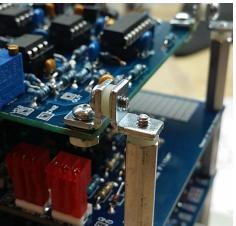
PCB; install a nut on the standoff threads there.
