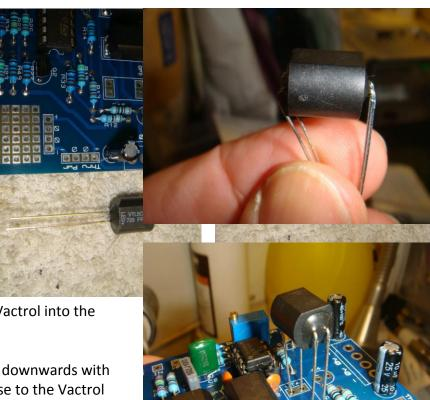
correct orientation for inserting the Vactrol into the PCB.
