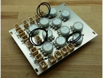
28. Now we will create crimped socket connectors and solder the wires to pots. The general process
